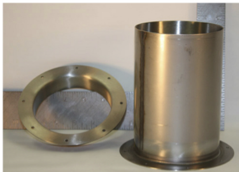
Air filtration sleeves and rings, 16 gage 304 s/s, ID polished to a #4 finish. 6" diameter od to 7" long.
