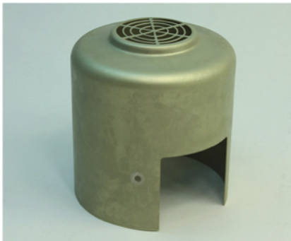
6061 Aluminum, chromate conversion anodize finish. Custom cover for a military motor. 5.00" diameter X 6.50" height x 0.040" thick aluminum formed using hydroforming.
